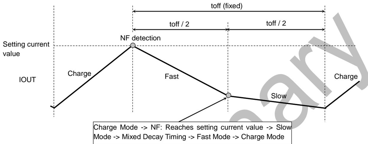
If the output current is zero-detected during OFF time, the output becomes High impedance.
