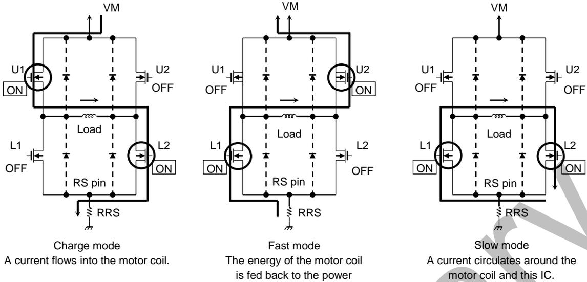
**Operation Function of Output Transistor**
